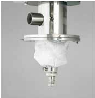
The top part of the spray consists of a liquid nozzle and an air nozzle.
