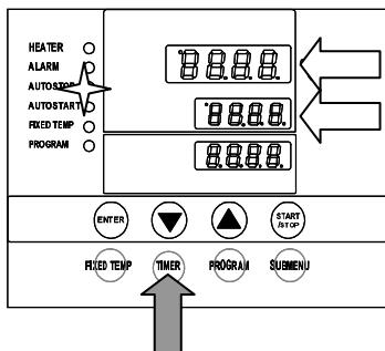
This operation is used to specify the automatic stop time in the fixed temperature operation.
