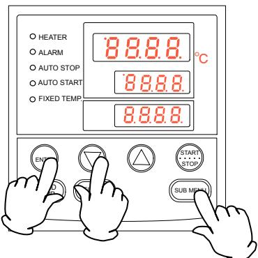
④ ③ To release lock, press the **Sub menu** key, select the characters **Lock** *Lock* that indicate the setting lock with the **▼▲** keys, and then press the **Enter** key. Select "OFF" with the **▼** key and then press the **Enter** key to release.
