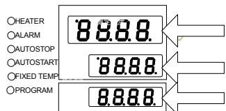
Measured temperature display : Displays the current temperature in the bath
