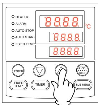
② "OFF" will appear on the set temperature display. You can lock the settings by setting to "ON" with the **▲** key.。
