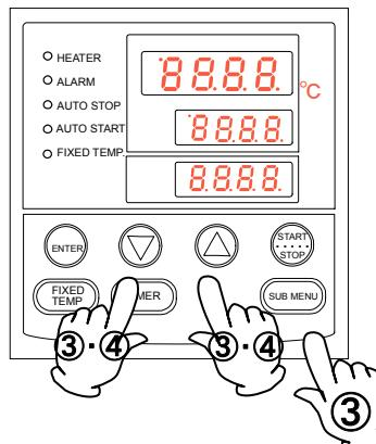
① Start operation at the target set temperature and check the in-bath temperature on a temperature recorder when the temperature is stable.
