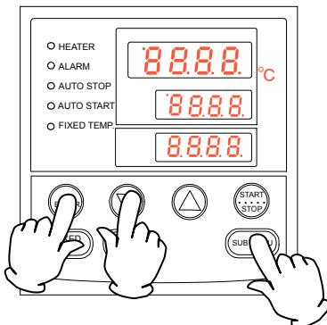
① Press the **Sub menu** key, select the characters **Lock** *Lock* that indicate the setting lock with the **▼▲** keys, and then press the **Enter** key.
