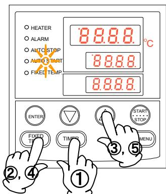
① On the initial screen, press the **Timer** key to blink the
