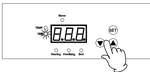
4. Press **▲** key to increase the time and press **▼** key to reduce it. After adjusting to the required time, press **SET** key another time to confirm the new setting and complete the time setting procedures. The sterilizing time may be set with reference to "Sterilizing Parameters" (p.14)
