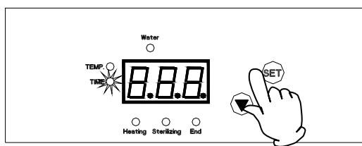
3. press **SET** key to shift the function lamp to the position of sterilizing time, and the time mode will be displayed. The sterilizing time may be set as required.
