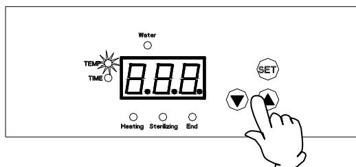
2. Press **▲▼** key to raise or reduce the temperature. After adjusting to the required temperature, press again to confirm the new setting and complete the temperature setting procedures.
