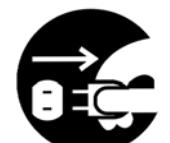
Compulsion disconnect the power plug
