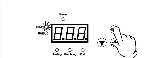
1. Press **SET** key to shift the function light to the position of sterilizing temperature, and now the display window will indicate the temperature mode. The sterilizing temperature may be set as required.
