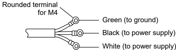
These models do not include the power plug. Correctly connect the ground to fit with the power supply facility to be connected.
