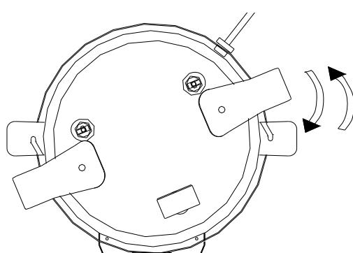
Note: the lid may only be opened after sterilizing finishes, the remaining steam is released till the pressure gauge indicates zero.
