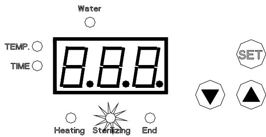
Note: After sterilizing, [End] display, the drain valve shall keep open, from which traces of steam will be exhausted to discharge the cold air in the pot, and the sample will be dried and sterilized completely.
