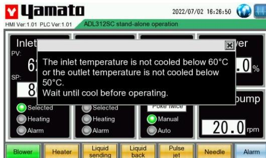
※ When the outlet temp. is above 50°C, do not stop the operation of the blower by forcibly cutting off the power. Otherwise, the malfunction may occur.
