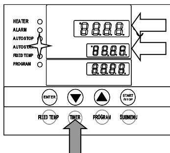
This operation is used to specify the period up to automatic start after power on.
