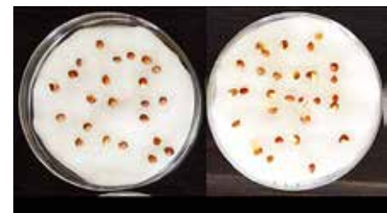
No plasma treatment plasma treatment 10 min
