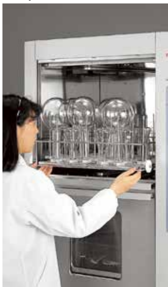
Jet cleaning frame (for AW83Z)
