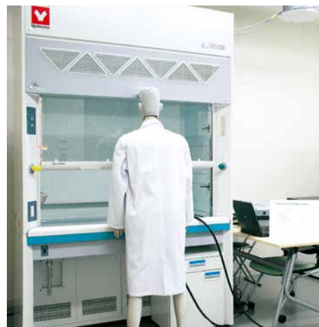
ASHRAE test fixed position test
