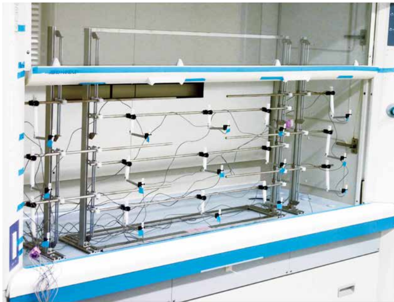
Multi-point anemometer wind speed measurement
