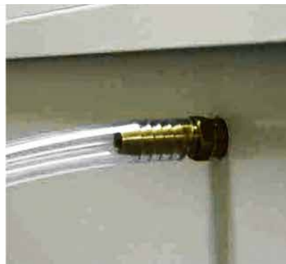
Dust collection efficiency measurement nozzle
