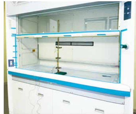
EN test wind speed measurement
