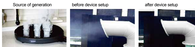
<Generation conditions> Heating temperature: 250°C Test reagent amount: 10 beakers with 100cc each
